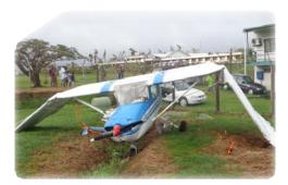
Additional safety measures could include placing chokes around the wheels, applying the parking brake and placing objects on top of the wings to reduce the lift generated by the airflow.
