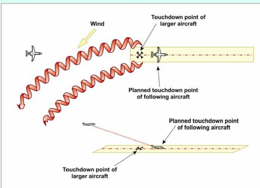
a. **Vortex Generation.** An aircraft generates vortices from the moment it rotates on takeoff to touchdown, since trailing vortices are a by-product of wing lift. Prior to takeoff or landing, pilots should note the rotation or touchdown point of the preceding aircraft (see Figure 4, Touchdown Points of Preceding and Following Aircraft).
