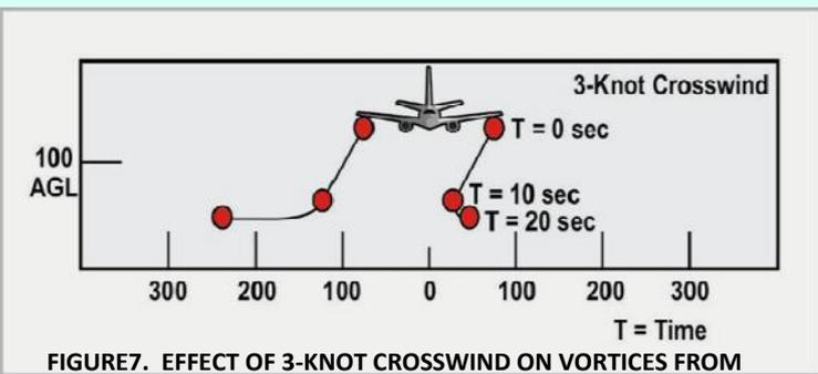
FIGURE7. EFFECT OF 3-KNOT CROSSWIND ON VORTICES FROM LOW FLYING AIRCRAFT
