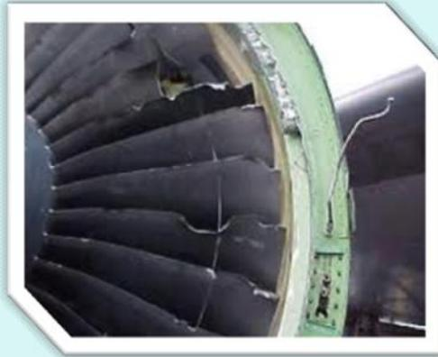
In December 2013, there were 3 confirmed bird strikes for Nadi – one of which caused \$36,000 worth of damage to fan blades on a Fiji Airways aircraft.
