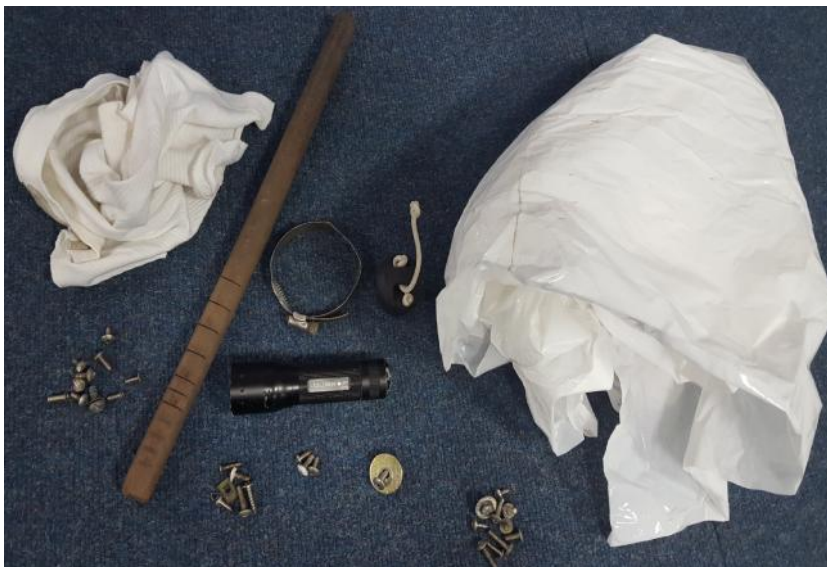
Figure 2. FOD items collected at Nadi International Airport; grease rag, fuel dip stick, torch, screws, an airline garbage bag, rubber plug and a hose clamp.
