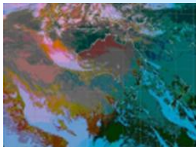
MTSAT-1R icing enhancement. Dark areas indicate the presence of supercooled liquid water (black by night, red by day). High Level cirrus (bright areas) may prevent the satellite from seeing the lower level clouds.
