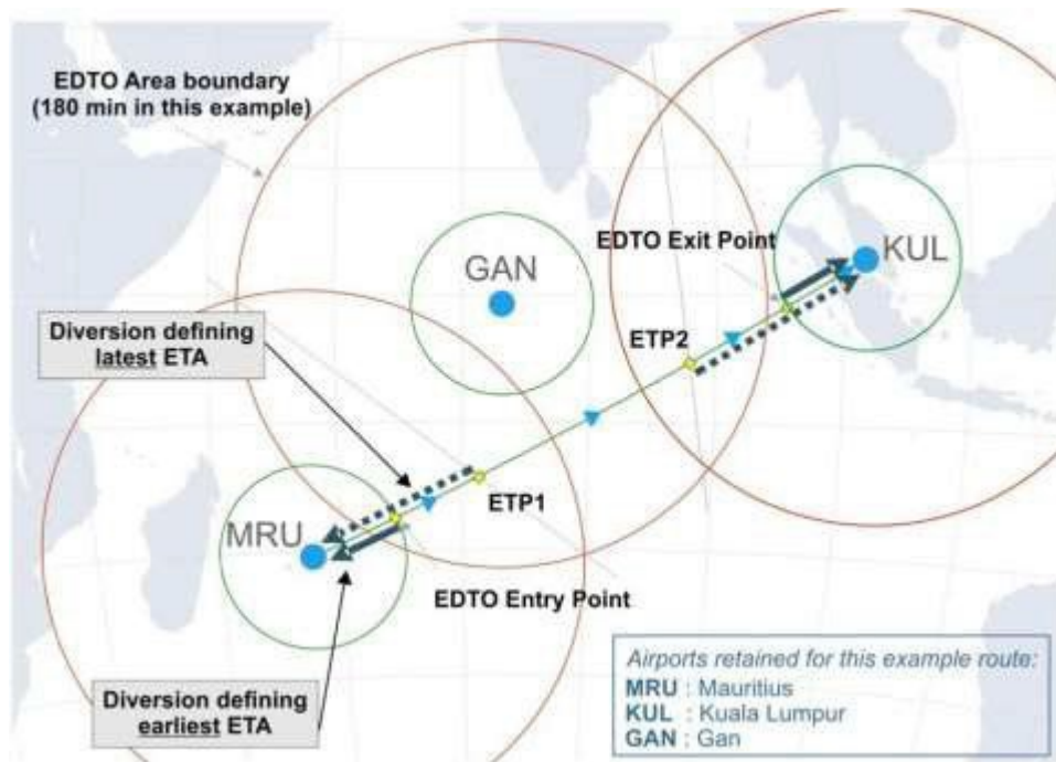
Figure 3.5-6b. Validity period of EDTO alternates located before or after the EDTO sector
