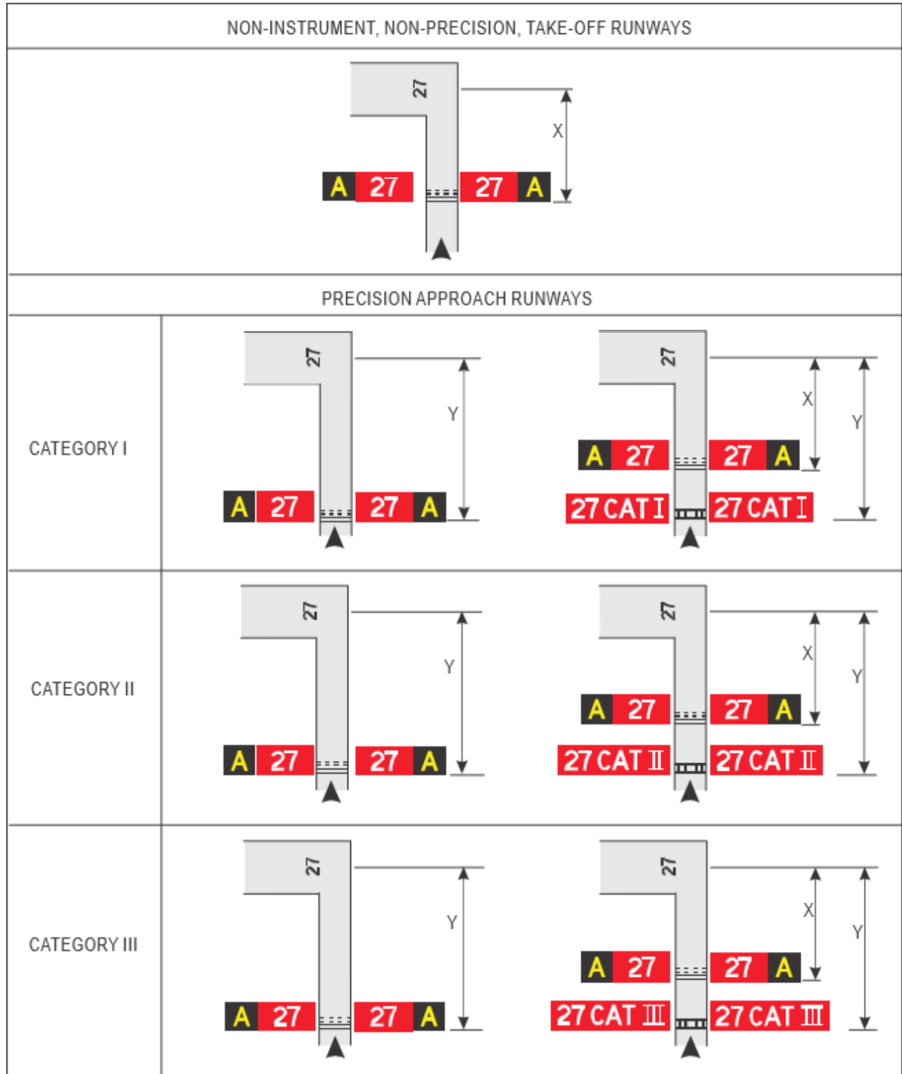
Figure 30 - Examples of sign positions at taxiway/runway intersections
